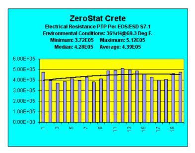
As shown, a properly installed ZeroStat Crete Monolithic Flooring System will post very consistent Point to Point Electrical Resistivity readings allowing the floor to comply with the latest specifications for even the most stringent of static control applications.
