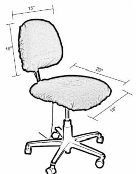
GZ's Dissipative Chair Cover turns regular chairs into ESD chairs. It's one size fits standard sized chairs and covers both seat and chair backs. The cover minimizes triboelectric generation, typically 10's of kilovolts on standard chairs. The fabric construction allows the fabric to breathe. The back and seat are electrically connected by a drag chain that completes the path to ground.
